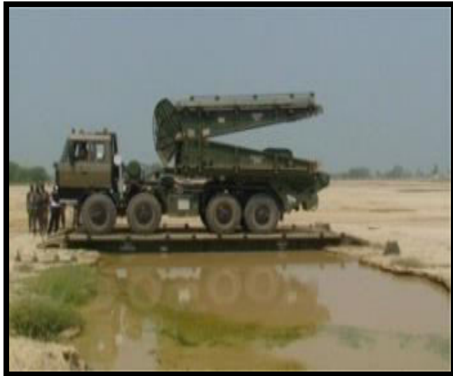
10 M SHORT SPAN BRIDGE
