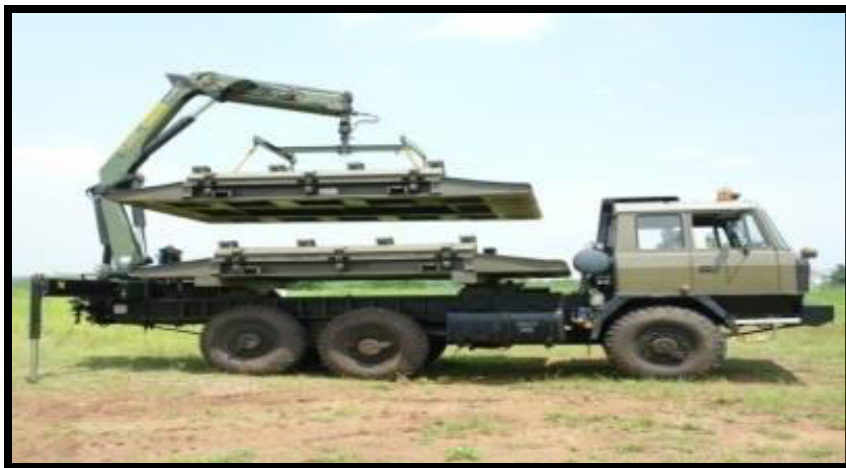
5 M SHORT SPAN BRIDGE
