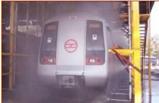
WATER TIGHTNESS TEST
