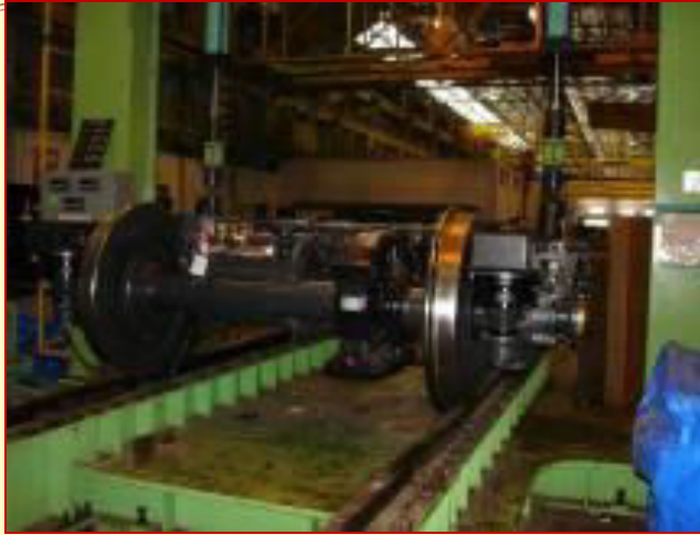
BOGIE LOAD TEST
