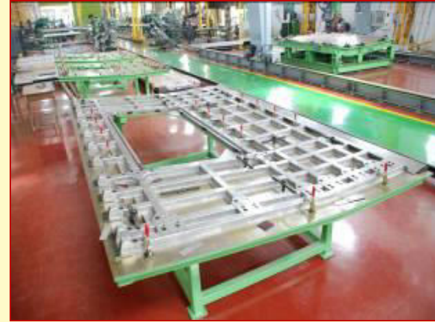
WELD JIGS FOR SIDE FRAME
