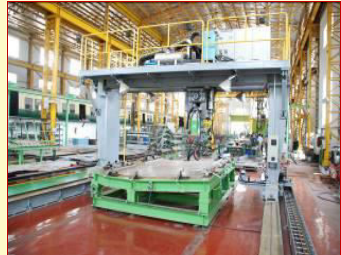
SERIES SPOT WELDING MACHINE FOR SIDE STRUCTURE
