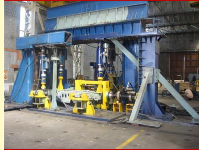
BOGIE FATIGUE & STATIC TEST
